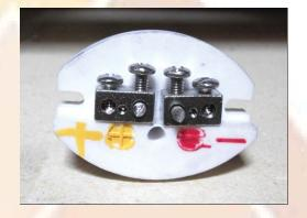
If you hook up the thermocouple incorrectly, your kiln or furnace will not operate properly. If your thermocouple is not marked, or if you believe it is incorrectly marked, you can check it with a magnet. The magnetic side is always the minus (-) and must be connected to the red wire.
