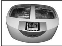
This sieve cleaner produces ultrasonic vibrations in a fluid bath which results in contaminants becoming dislodged from the sieve frame and cloth. Cleans one 8" (200 mm) diameter full height stainless steel or brass test sieve at a time.
