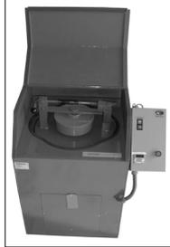
Application: Wet or dry pulverizing of minerals, ore, rock, soil, sand, slag, coal, coke, glass and similar materials to analytical fineness of 100 to 400 mesh from an original size of 1/2" or more. Features sound damping enclosure with anti-noise lining, and timer for cycle selection.
