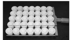
Overall length 58". Forks for #7 cupels can also be used with #6A, 7A, SA, 7X, and other 1-9/16" and 1-1/2" cupels. Forks for #8 cupels can also be used with #8A, 8AM, and #8S.
