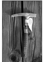
Estwing Leather Grip Rock Picks - 22 ounce head with polished head, shank, and pointed tip. Forged one piece head and handle. Brown laminated leather grip. The sole-leather washers are pressed on and riveted.
