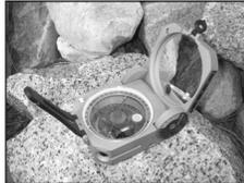
Geo Pocket Transit features a solid aluminum case and a fast, magnetic north seeking, rare-earth magnet. Also includes a hinge inclinometer, accurate to +/- 2°. This feature allows simultaneous trend and plunge measurements, reducing the number of measurements required in the field. Needle can be locked or unlocked and feature a lift-pin, are waterproof and international.
