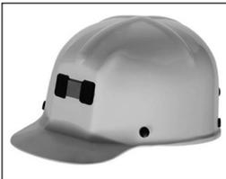
Molded cross ridges on the crown provide increased strength and rigidity. The cap's peak helps protect the wearer's eyes and face from small falling objects. Not designed to protect against lateral blows from the front, side or rear.
