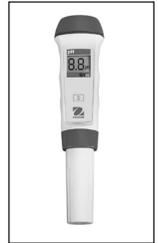
**pH Pocket tester pH55:** Waterproof pH tester with large dual-level LCD that displays pH and temperature (C or °F). The display shows readings in an extended range from -2.0 to 16.0 pH and simultaneously shows temperature. 0.1pH resolution.
