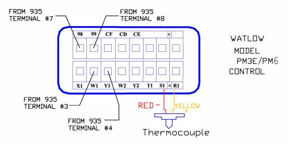
\*NOTE-BE SURE ALL WIRING CONNECTIONS ARE CORRECT BEFORE APPLYING POWER! THE WARRANTY DOES NOT COVER DAMAGE DUE TO INCORRECT CONNECTION.
