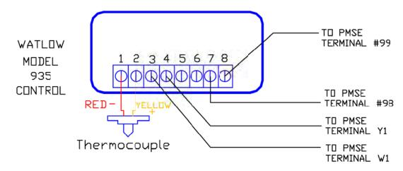
TRANSFER ALL WIRES FROM THE OLD CONTROL TO THEIR CORRASPONDING CONNECTIONS ON THE NEW CONTROL UNLESS OTHERWISE NOTED.
