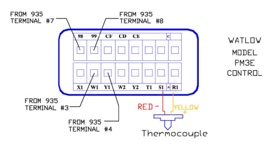
\*NOTE-BE SURE ALL WIRING CONNECTIONS ARE CORRECT BEFORE APPLYING POWER! THE WARRANTY DOES NOT COVER DAMAGE DUE TO INCORRECT CONNECTION.
